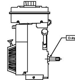
5. Place the back plate (3) on the engine, checking a close fit between the back plate and engine flange. Before fixing the parts, be sure that the position of the back plate is correct with the nameplate place up.
